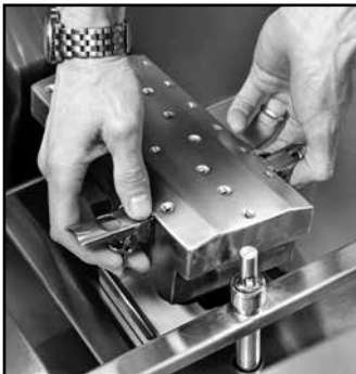
Spray box Spray box gasket (located under spray box - not shown)
